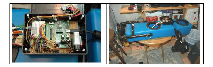
Here are pictures with the access hatches removed. The picture on the left is where the BS2 is mounted. The picture on the right is where the motor controllers are mounted, note, I also added LED's on the motor controller box to indicate each motor's direction.
