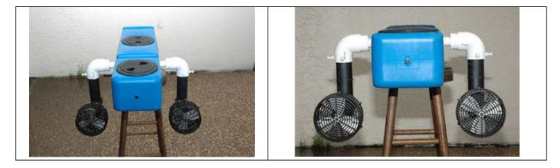
The next step was to build the "sensor pack", this is the PVC framework where the "whisker switches" and infrared detector will be mounted. Once again, the original molded-in nuts in the hull were utilized
