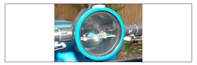
The second set of sensors are "whiskers" which are made by attaching a bent piece of wire from the hobby store between two momentary lever switches. Each set of switches are wired together to create one big switch. A whisker is mounted on each side to provide feedback if the SWIMMER touches the pool wall.
