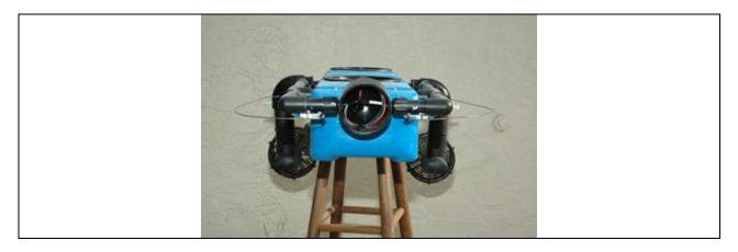
For the debris intake, I used an attachment from a shop-vac that is connected to a 3" piece of PVC and ultimately empties into a net bag that is mounted in the rear. There is no vacuum, the forward motion is enough to guide the debris into the intake and therefore into the net bag.
