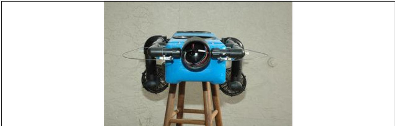
For the debris intake, I used an attachment from a shop-vac that is connected to a 3" piece of PVC and ultimately empties into a net bag that is mounted in the rear. There is no vacuum, the forward motion is enough to guide the debris into the intake and therefore into the net bag.
