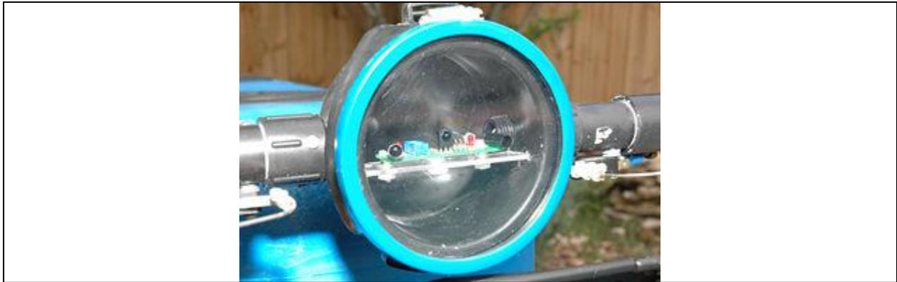
The second set of sensors are “whiskers” which are made by attaching a bent piece of wire from the hobby store between two momentary lever switches. Each set of switches are wired together to create one big switch. A whisker is mounted on each side to provide feedback if the SWIMMER touches the pool wall.
